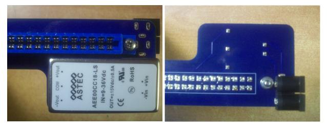
If the optional PSU is not used, bridge the "208 supply" pads to the right to power the Hub's +/-15V rails with the 208's ones, with headers + jumpers or solder components legs.
